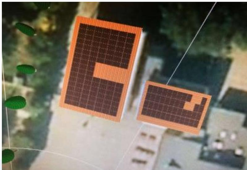
Solar panels will be installed at the Essex Outdoor Centre that will produce around 21,000 kWh of electricity in their first year. That's around the same amount of electricity needed to supply seven average homes. Essex County Council is also looking at other building at the Essex Outdoor Centre that would be suitable for installing solar panels on.
